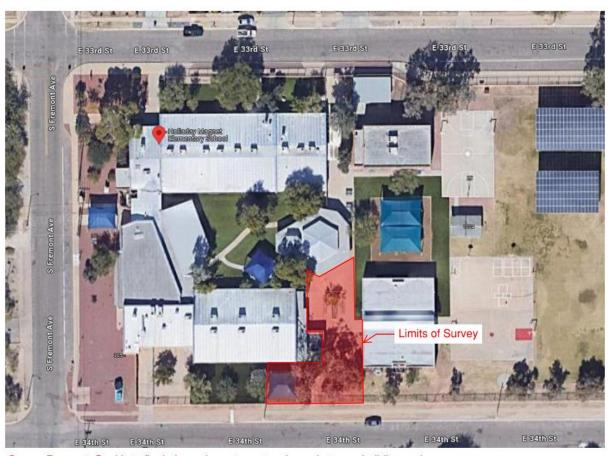
Survey Request: Goal is to fix drainage in east courtyard area between building and stairs. Please pick-up detailed survey at every concrete joint and stair. Need 0.5-foot contours and any existing culture.
